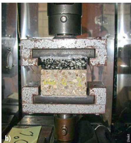
Photos 3 Dispositifs de cisaillement direct (a) et de traction directe (b) disponibles au CRR Direct-shear (a) and direct-tensile (b) strength testing devices available at French road research centre (CRR)
